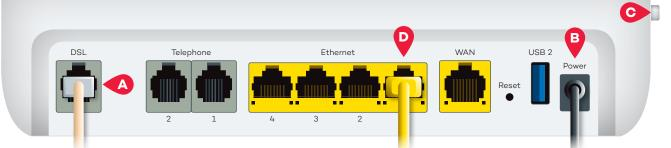
Connect the supplied RJ-11 cable to the DSL port on the back of the router and to the phone port that supplies your DSL service.
